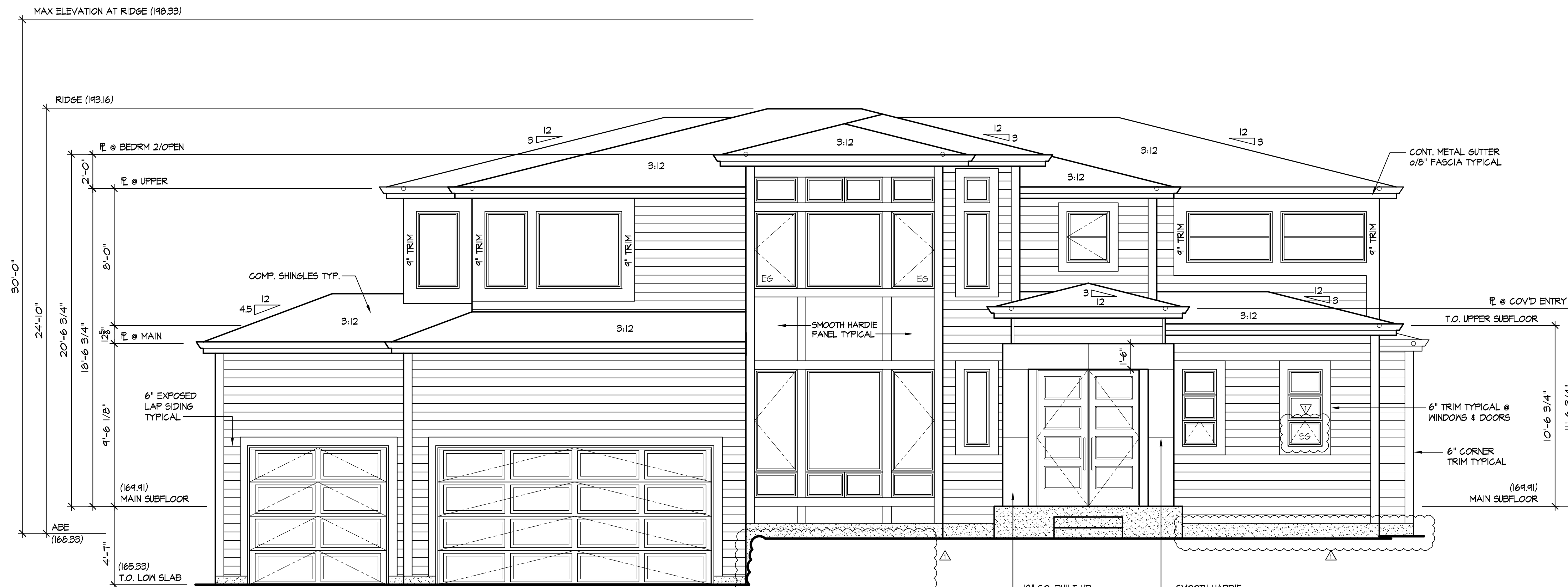
NORTH ELEVATION SCALE: 1/4" = 1'-0"
